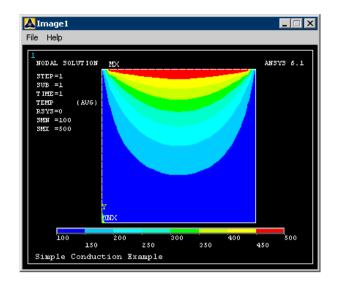
**Result**: Steady state heat transfer Analysis on Axisymmetric component is done.
