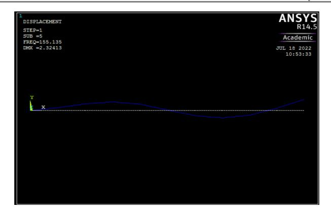
**Result**: Natural frequencies and mode shapes of 2-D Beam are done.
